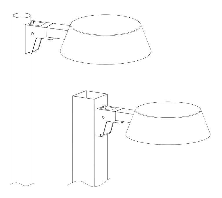
**Notes:** Do not energize luminaire until installation is completed. General contractor is responsible for providing appropriate anchoring devices to support load of fixture.
